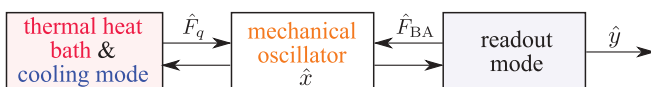
FIG. 2. (Color online) The relation among different parts of the optomechanical system in the experiment. The thermal heat bath and the cooling mode together create an effective quantum heat bath for the mechanical oscillator, which in turn couples to the readout mode.
