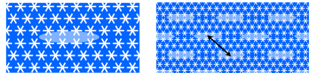
FIG. 1: A planar slab of silicon with a periodic arrangement of snowflake-shaped holes (here viewed from above) forms a two-dimensional optomechanical crystal. (Left) By disrupting the alignment between successive horizontal lines and (not visible) locally altering the structure along that linear defect, Safavi-Naeini et al. produced a single localized defect mode (indicated here by a shaded ellipse) for optical radiation at the same place as a localized vibrational mode of the structure. (Right) In the future, a periodic arrangement of such defects could produce an “optomechanical array,” with photons and phonons tunneling between each pair of neighboring sites (exemplified by the arrow) and interacting with each other. (APS/Florian Marquardt)
