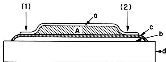
FIG. 1. Cross section of a Josephson junction pair vacuum-deposited on a quartz substrate ( $d$ ). A thin oxide layer ( $c$ ) separates thin ( $\sim 1000\text{\AA}$ ) tin films ( $a$ ) and ( $b$ ). The junctions (1) and (2) are connected in parallel by superconducting thin film links forming an enclosed area ( $A$ ) between junctions. Current flow is measured between films ( $a$ ) and ( $b$ ).
